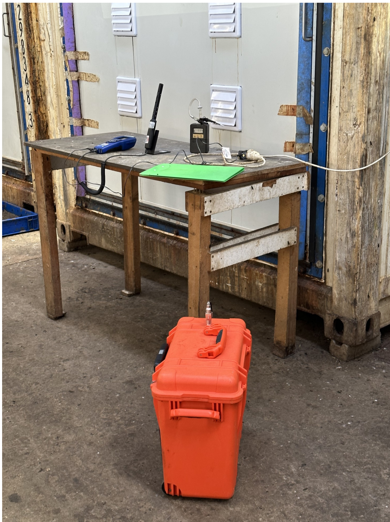
Figure 23 Air sampling for CO 2 , VOCs and odour
